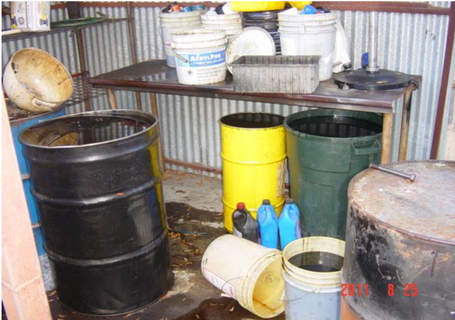
Open containers and drums full of used oil observed at northwest side of property. This area is being used as the hazardous waste storage area.
