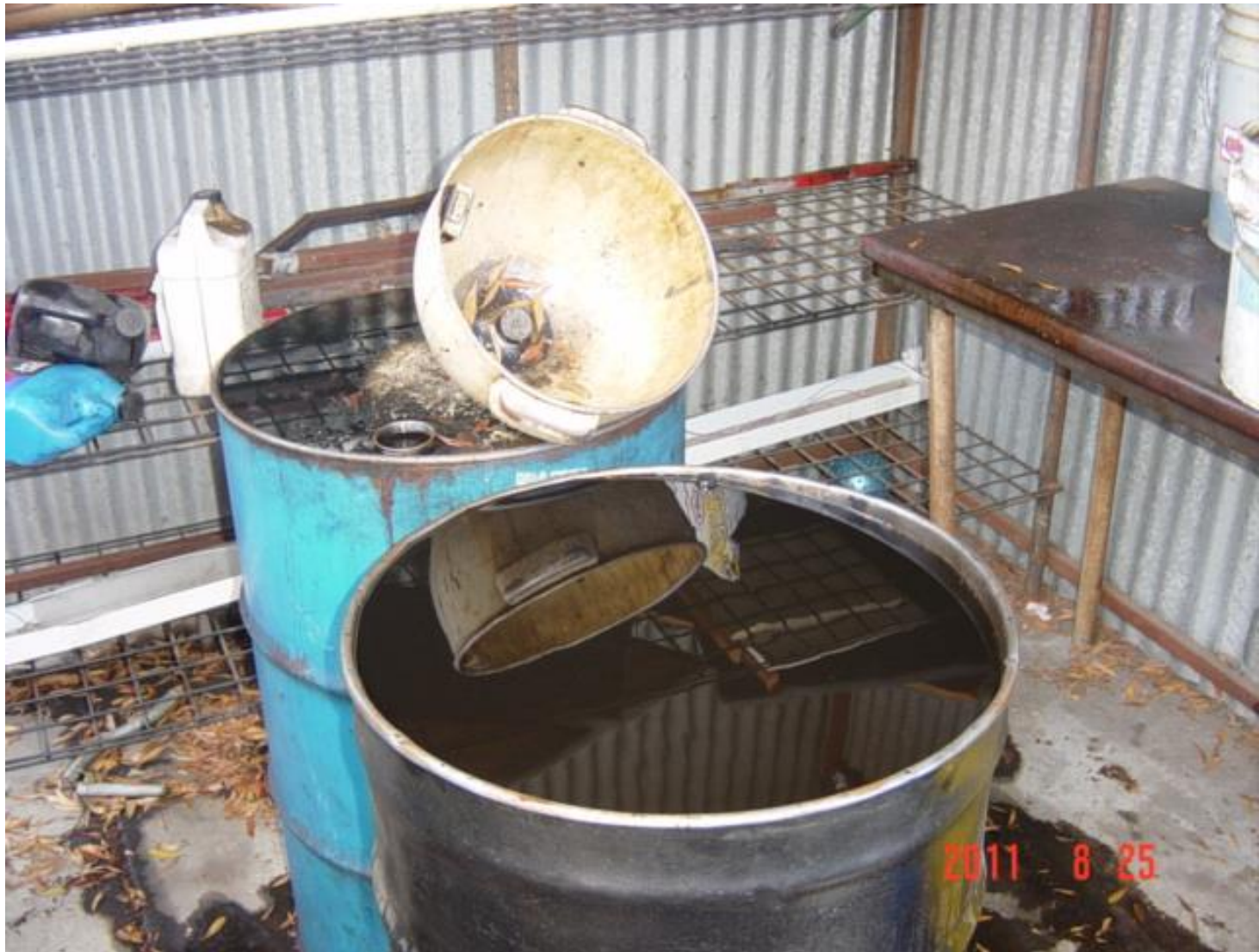
Close-up of 55gal drum with open top and 55gal drum with open bung hole. Both drums were observed to be 100% full of used oil. Evidence of used oil spillage due to overflowing containers was observed as well.
